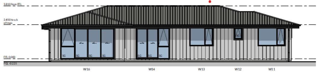
NORTH ELEVATION Scale 1:100 @ A3 SG = Safety Glazing
